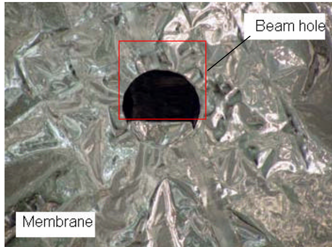
Fig. 5.18 Picture of the membrane at the entrance of the beam hole.
